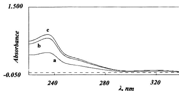
Fig. 2. Zero-order absorbance spectra of bromazepam in, (a) buffer solution of  $\text{NaH}_2\text{PO}_4$  0.1 M (pH 7.0); (b)  $\beta$ -hydroxypropylcyclodextrin (pH 7.0) and (c)  $\beta$ -CD (pH 7.0). The above solutions were prepared by weighing 0.0032 g of bromazepam, diluting to 10.0 ml with buffer solution or cyclodextrin solution  $1.3 \times 10^{-2}$  M, buffered at pH 7.0, shaking for 24 h, filtration through filter papers and final dilution 1:25 with buffer solution.
