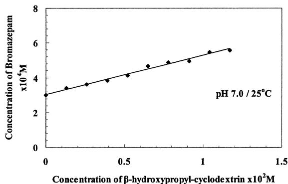
Fig. 3. A typical phase solubility diagram of an inclusion complex of bromazepam with  $\beta$ -HP-CD at pH 7.0 and  $\theta = 25^\circ\text{C}$ .
